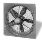
Square plate mounted axial fan with highly efficient impeller, dynamically balanced to DIN ISO 1940 and VDI 2060 class 6.3, manufactured from impact resistant anti static polymers. Suitable for -30°C to +40°C. Fitted with motorside guard. Explosion Proof II 2G C IIB T3 Gb according to ATEX. Totally enclosed, three phase motor. Maintenance free with low-noise sealed for life ball bearings.
